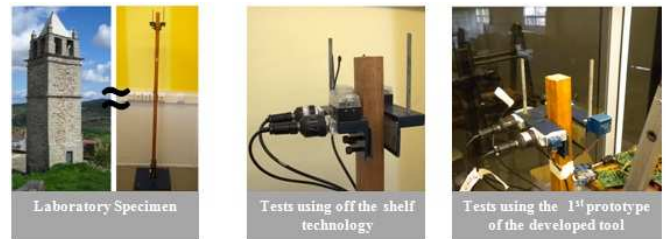
Fig. 7. Laboratory system idealization/experimental setups
