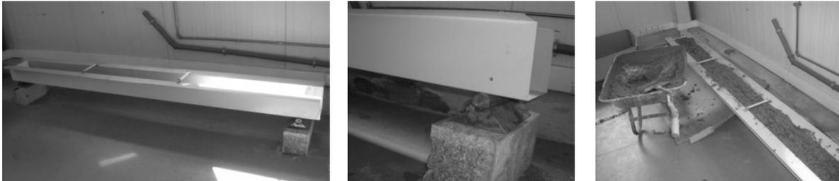
Figure 6.11 – Details of the steel formwork used for the tests of the CB-01 and CB-02 and the concrete casting process
