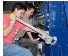
Figure 5.26 – Experimental tests in the tie-rods: (a) scheme of the test; (b) laboratory setup; and (c) LVDTs arrangement and application of the tensile force
