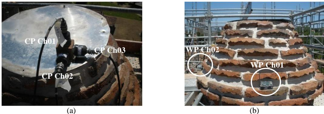
Figure 4.26 – Modal identification tests in the Chimneys at Paço dos Duques building: (a) conventional accelerometers' arrangement; and (b) WSN platforms' arrangement
